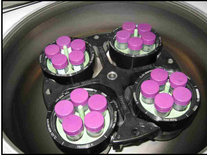
Figure 3.4 20 mL of Solutions Were Centrifuged for the Solid/Liquid Separation Using Sorvall Legend RT
