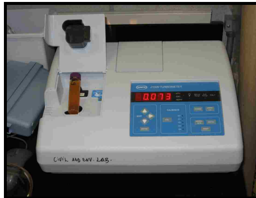
Figure 3.5 Turbidity Was Measured Using a 2100N Hach Turbidity Meter
